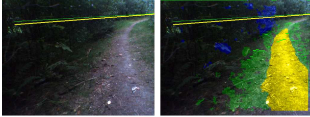
Fig. 9. Example of path classification. The costmap in Fig. 10 was created by driving along this path. The yellow color indicates the detected path. Green is ground plane and blue are obstacles. The two horizontal lines are estimates for the location of the horizon.
