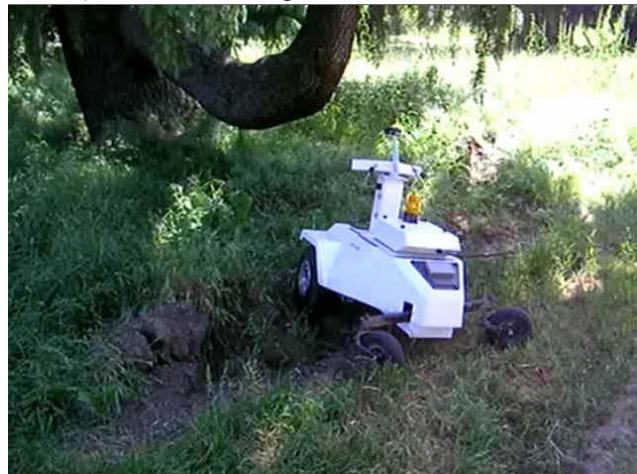
Figure 6 Outdoor robot in typical terrain. Robot is part of a DARPA project, Learning Applied to Ground Robotics. Two stereo systems are on the upper crossbar.
