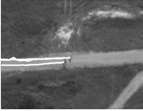
Figure 2: Synopsis of a video of people running, with detected tracks in white. The ground is basically flat, and the images of the people are about 15 pixels high.
