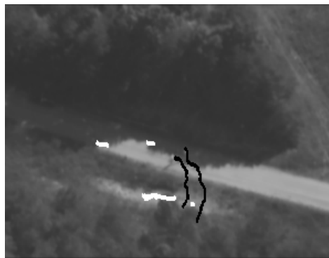
Figure 1: An example of parallax artifacts in airborne video. This is a frame showing a road cutting through woods with tracks of detected objects overlaid. People crossing are in black and artifacts generated by trees are in white.
